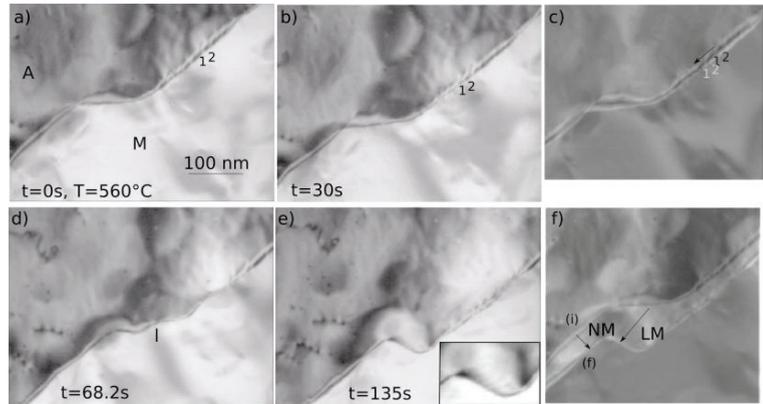
Fig.2. Ledge motion of the austenite/martensite interface. Displacement of interfacial dislocations are seen (1, 2) (a-c). f) is the image difference between a) and e) showing both ledge motion (LM) and normal motion (NM).
