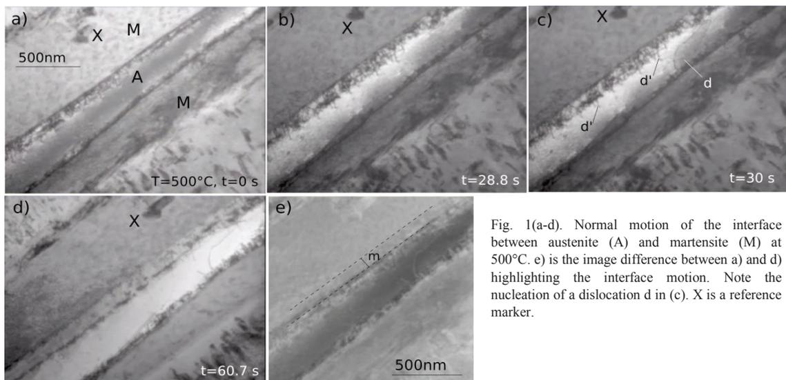
Fig. 1(a-d). Normal motion of the interface between austenite (A) and martensite (M) at 500°C. e) is the image difference between a) and d) highlighting the interface motion. Note the nucleation of a dislocation  $d$  in (c). X is a reference marker.
