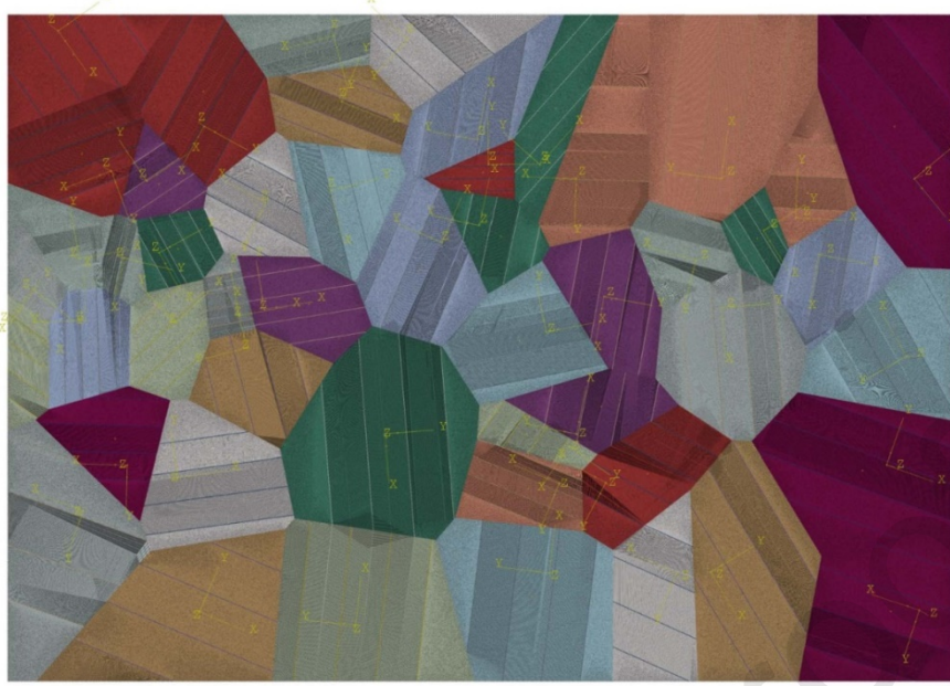
Figure 28. Finite element mesh of an aggregate containing 50 grains with four channels per grain. Each grain is colored differently with channels seen as narrow, parallel bands within each of the grain.
