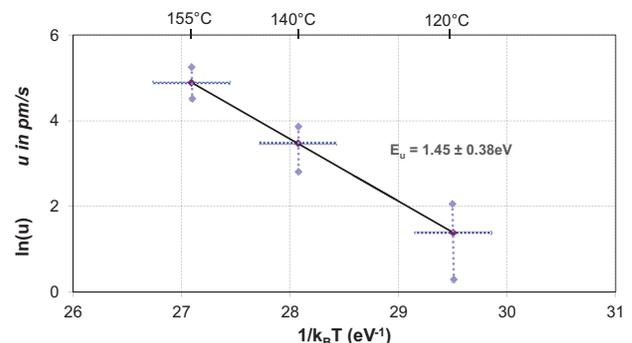
FIG. 2. (Color online) Activation energy for growth extracted from the slope of the Arrhenius plot (Eq. (1)) dotted lines represent error bars.
