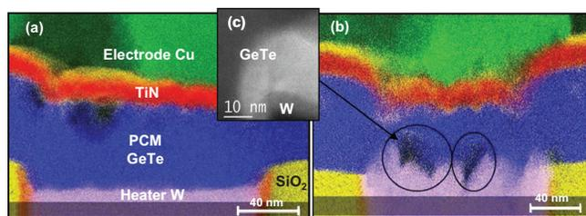
FIG. 3. (Color online) STEM-EDS maps of GeTe devices after (a) one amorphization and (b) after  $10^7$  cycles. Contrast colors correspond to the different elements of the device. (c) HREM image taken of the dark region encircled in (b).
