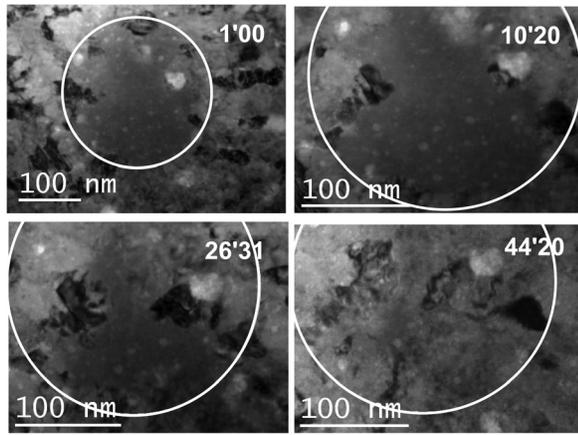
FIG. 1. TEM bright field images selected from the *in situ* crystallization sequence of the GeTe “melt quenched” spot at 155 °C.
