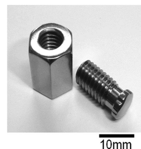
Figure 35. A set of pure Ti bolt and nut with the harmonic structure.
